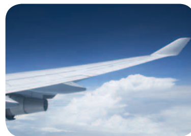
Fuji Heavy Industries used Optimus to automate and couple FEM and CFD simulations to identify optimized aircraft winglet design configurations. Optimus realized a 1.2% reduction in aircraft takeoff weight for a typical mission profile at 1G cruise speed.
